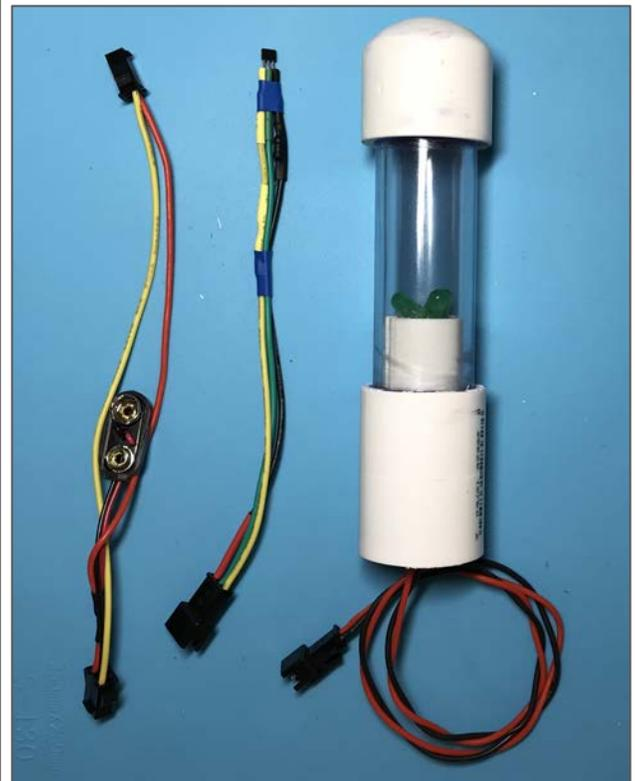
*Figure 1.12. Example Using JST Connectors*
