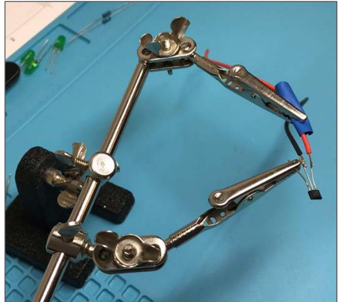
*Figure 1.15.* Example of securing components using grippers.
