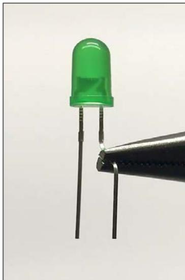
Figure 2.16. 2<sup>nd</sup> Bend – Front View
