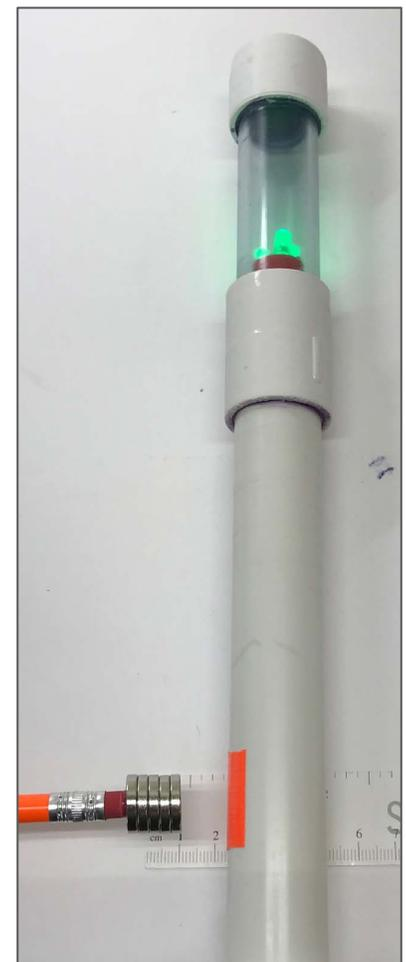
**IMPORTANT NOTE:** For successful activation, the magnet's South pole must be facing the Hall Effect Sensor.
