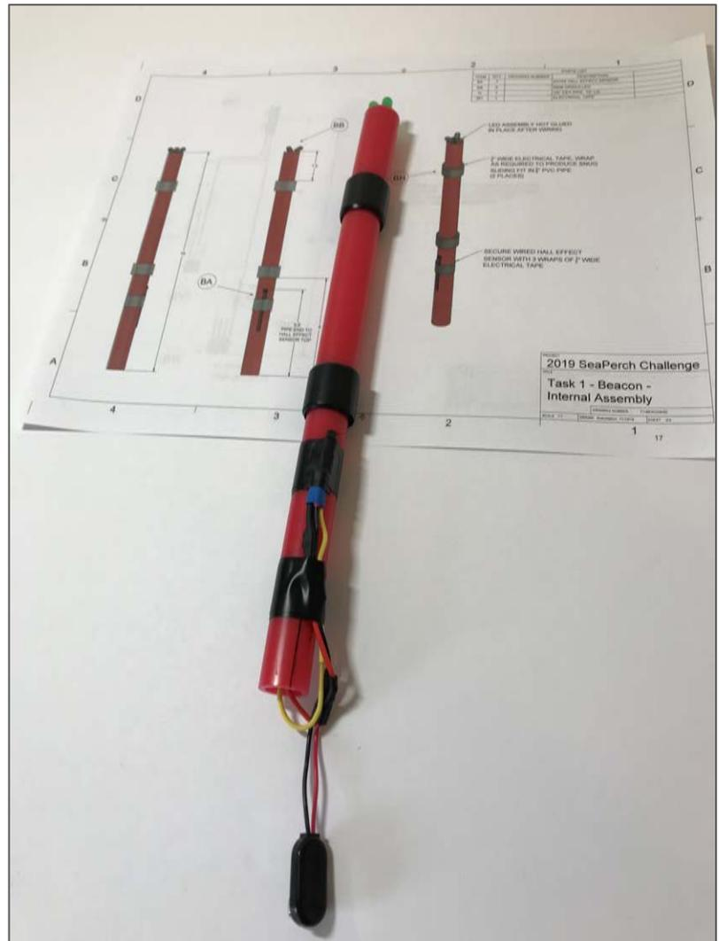
Figure 3.1. Completed Beacon Internal Assembly
