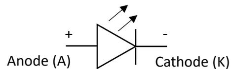
Figure 1.8. LED Electronic Circuit Schematic Representation
