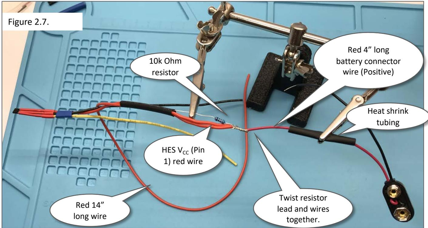
9. Place heat shrink tubing on wires **prior** to soldering.
