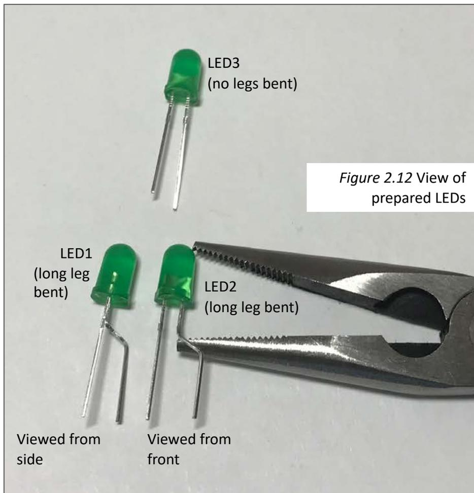
Figure 2.12 View of prepared LEDs
