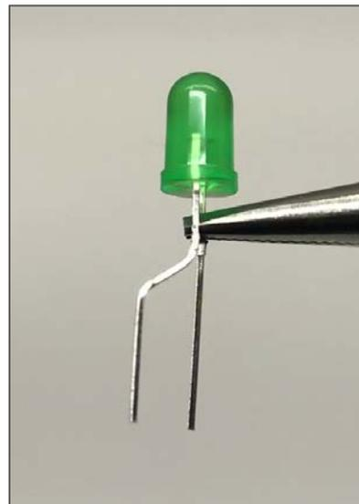
Figure 2.17. 2<sup>nd</sup> Bend – Side View
