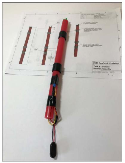
Figure 3.1. Completed Beacon Internal Assembly
