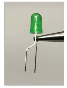
Figure 2.17. 2<sup>nd</sup> Bend – Side View
