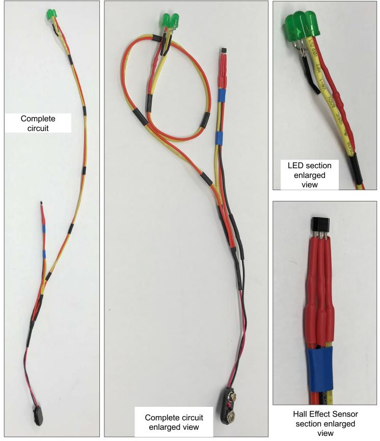
Figure 2.24. Completed Beacon Circuit (various views)
