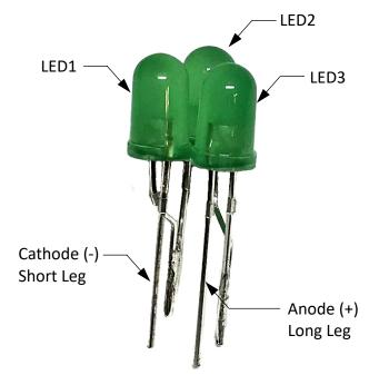
Figure 2.11 Completed LED Array
