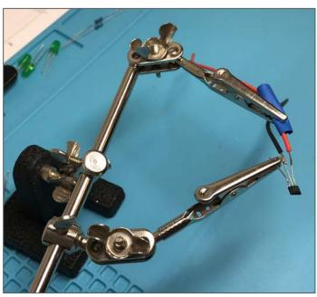
*Figure 1.15.* Example of securing components using grippers.
