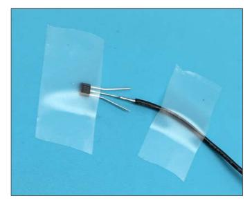
*Figure 1.14.* Example of securing components using tape.
