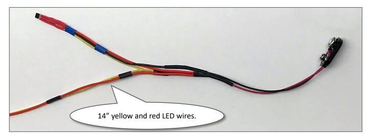
Figure 2.10. Completed Hall Effect Sensor/Power Cable with LED Wires
